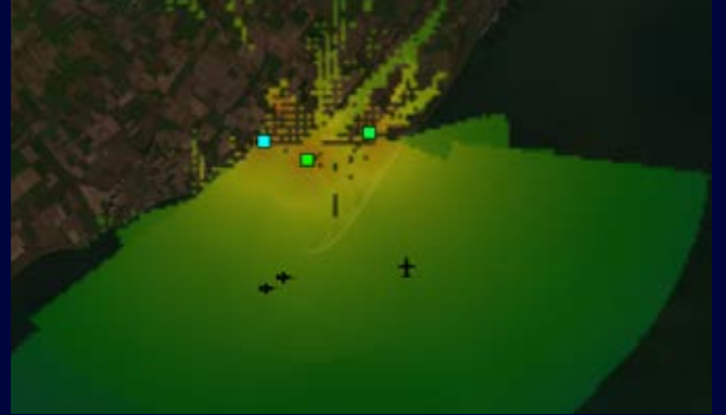
Image 9: A relief map with a sensor network comprising four RFeye Nodes. The heatmap shows free space RF propagation, with yellow indicating good signal quality, and green indicating fair signal quality. Signals that have been identified and geolocated by RFeye Site are represented by icons.
