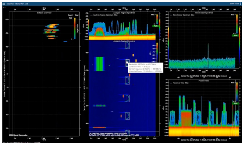
>>> Image 1: When hovering over the signal, Signal Discovery shows the pulse descriptor
